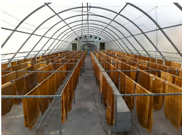
Fig. 3. The pictorial view of greenhouse solar dryer with natural rubber sheets inside (Jitjack et al., 2016).
